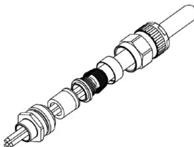
Figure 13. Example of cable gland
